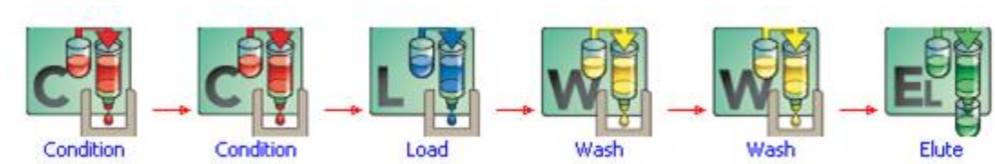
Figure 3. TRILUTION® LH Basic SPE Tasks for Solid Phase Extraction of Patulin from Apple Juice
