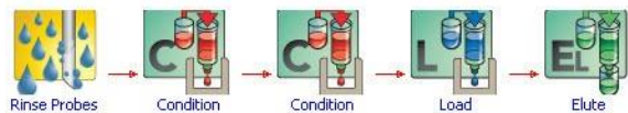
Figure 2. TRILUTION LH Basic SPE Tasks for Solid Phase Extraction of Lamotrigine and Metabolite from Water
