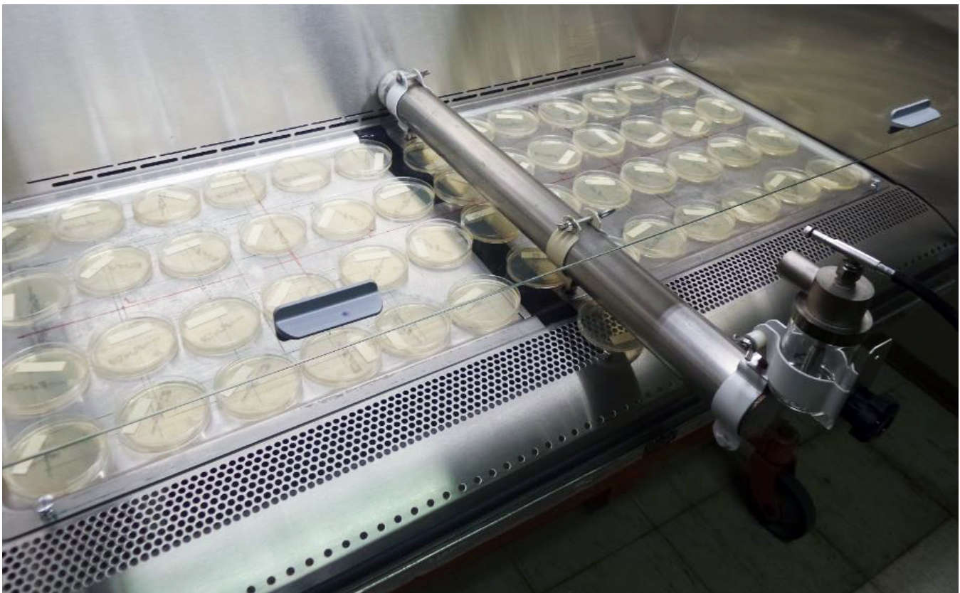
Microbiological challenge testing on an NSF listed Class II, Type A2
