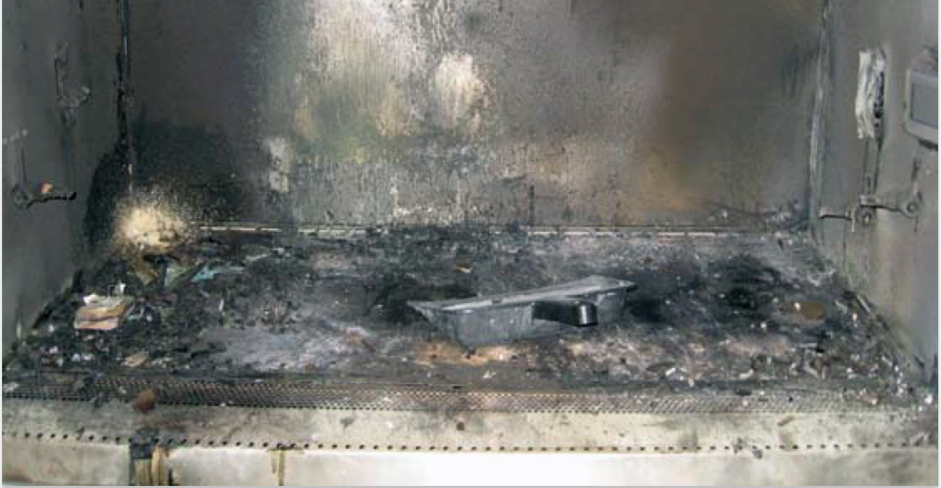
BSC with fire damage
