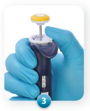
push the thumbwheel down to lock it and start pipetting!
