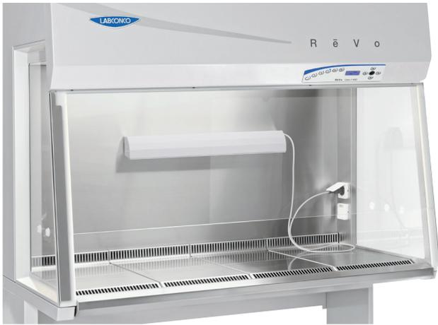
**R3858500—Ultraviolet Lamp Kit.** Magnetically attaches to rear wall of ReVo and ReVo Pro cabinets for secondary cabinet disinfection. Includes 254 nm UV lamp with power cord. **Installation required.**
