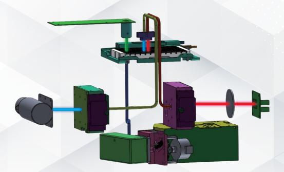
INNO-S<sup>M</sup> has three main detecting functions. Since INNO-S<sup>M</sup> is a monochromator-based microplate spectrophotometer for the absorbance measurements, it requires zero filters and allows you to measure from 200 to 999 nm freely at your choice of 1nm increment. Also Xenon lamps in absorbance will serve the instrument semi-permanent life time which brings the comfortable experiences to the users since the lamps do not need to be replaced such as halogen lamps.
