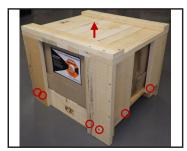
1. Unscrew 12 screws at the bottom of wooden crate. 6 screws are marked on above picture with circles, other 6 screws are located at the same positions on the other side of the crate. Then remove the upper part of the wooden crate by lifting it.
